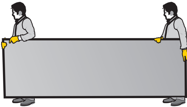
Figure 1 - LAMINAM® slab dimensions 1,000 x 3,000 mm
