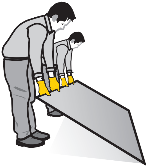
Figure 4 – Intermediate slab lifting phase
