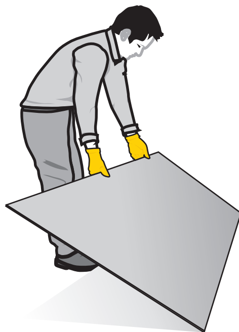
Figure 8 – Intermediate slab horizontal positioning phase
