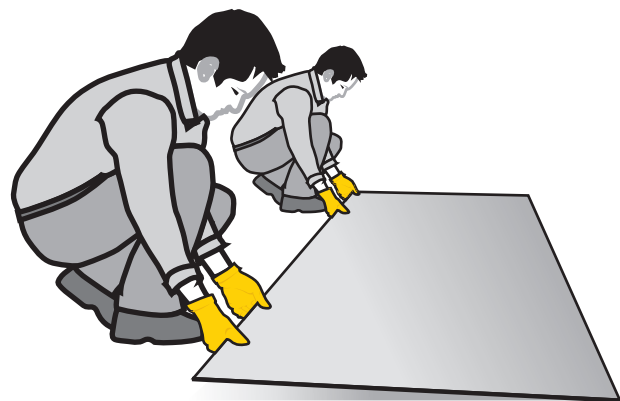
Figure 3 - Initial slab lifting phase
