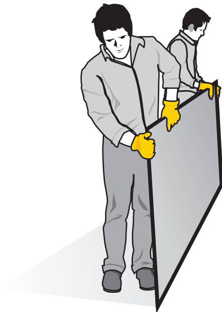
Figure 5 - Final slab lifting phase to vertical position
